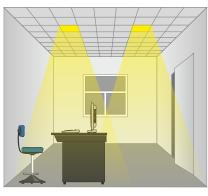
Micrprismatic lampshade (diffuser) of which are equipped with LED lamps Lumax Panel of professional series provides glare control. UGR (Unified Glare Rating) determines how much light disturb performing specific tasks. This is especially important in the workplace, where tasks such as reading, writing, computer work, precision assembly are doing, but also in conference or lecture rooms.
