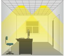
Standard milky lampshade 120° provides a wide Lambertian light distribution, which is suitable for spaces that require lower intensity lighting as well as other places where are carried out simple visual tasks. Wide beam angle lets reduce the number of luminaires at the design stage.
